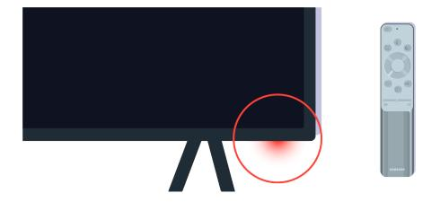
Check the remote control sensor again. If the LED is turned on, press the power button on your remote control to turn on your TV.
