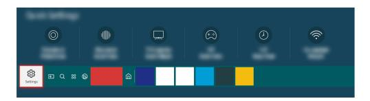
Check the volume on the screen. If a number for the TV volume is not displayed, select O > B Settings > Sound > Sound Output. Then, select TV Speaker.
