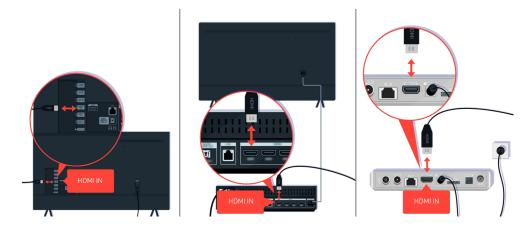
Check the antenna and HDMI cable connections.
